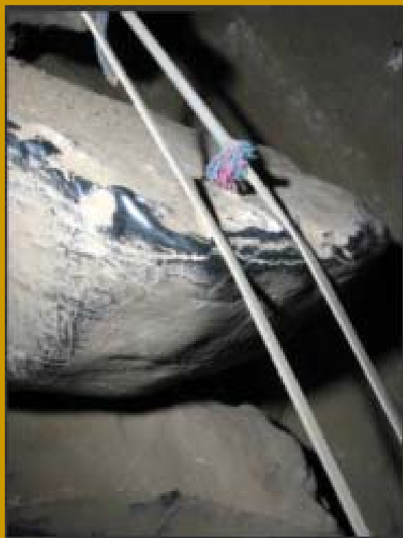
A fixed rope with worn sheath
